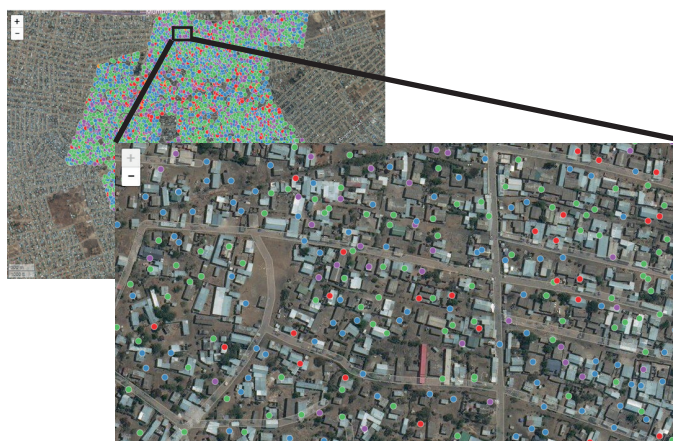
Figure 1: Kanyama's pit latrines - located and colour coded according to fullness. Red = full pit latrine, blue = almost full, green = half full, purple = almost empty, yellow = empty. Source: mWater.
